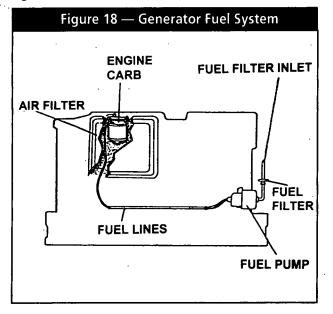
DANGER: GASOLINE IS HIGHLY FLAMMABLE AND ITS VAPORS ARE EXPLOSIVE. COMPLY WITH ALL CODES, STANDARDS AND REGULA-TIONS PERTAINING TO GASOLINE FUEL SYS-TEMS USED IN INDUSTRIAL MOBILE GENERA-TORS. PROPERLY INSTALL AND MAINTAIN THE FUEL SYSTEM AND KEEP IT ENTIRELY FREE OF LEAKS. GASOLINE VAPORS MUST NOT ENTER THE VEHICLE INTERIOR.
